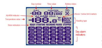
Pressing the review button, will display the current day's statistics, showing the Maximum temperature first, then the minimum temperature. Each press of the review button will display the maximum and minimum for each subsequent day. To return to the normal screen, press the start button once. The display will revert to normal mode if no buttons are pressed for 30 seconds
